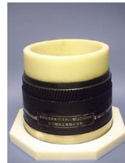
Figure 6 Photo of water suction pipe using PE-100.
