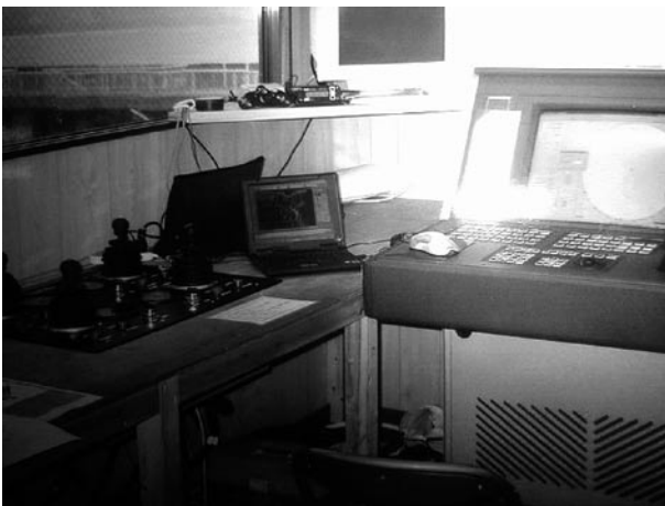
Figure 14 Control stand of barge with onboard DPS.
