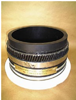
Figure 4 General structure and photo of large-diameter water suction pipe.
